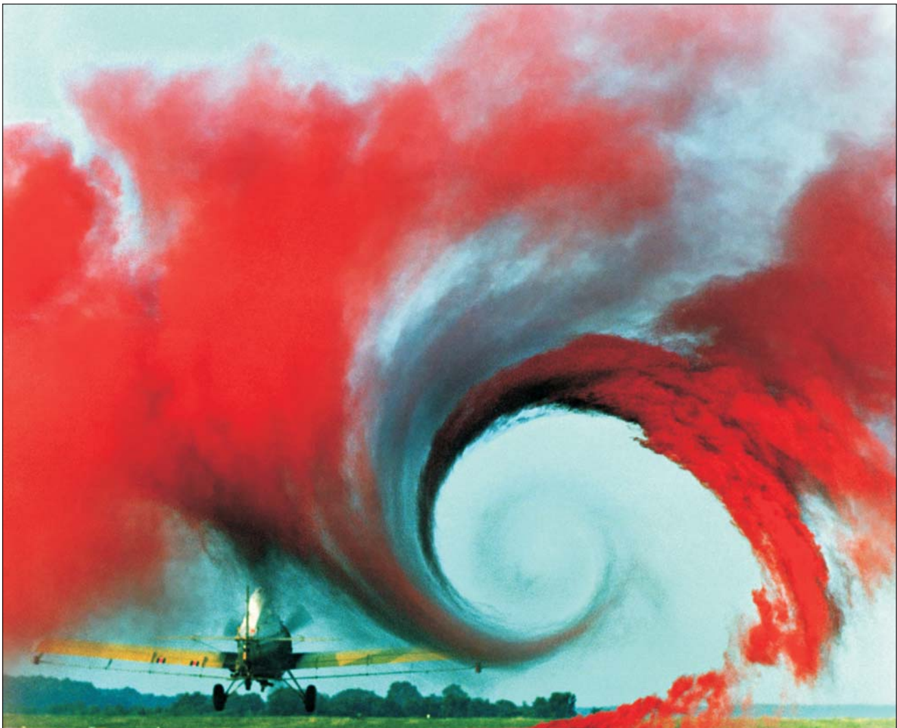
A NASA wake turbulence study at Wallops Island in 1990. A vortex is created by passage of an aircraft wing, revealed by smoke. Vortices are one of the many phenomena associated with the study of aerodynamics. Photo via Wikimedia Commons. [Public domain.]
