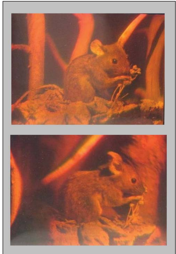
Two photographs of a single hologram taken from different viewpoints. Photo via Wikimedia Commons. [Public domain.]
