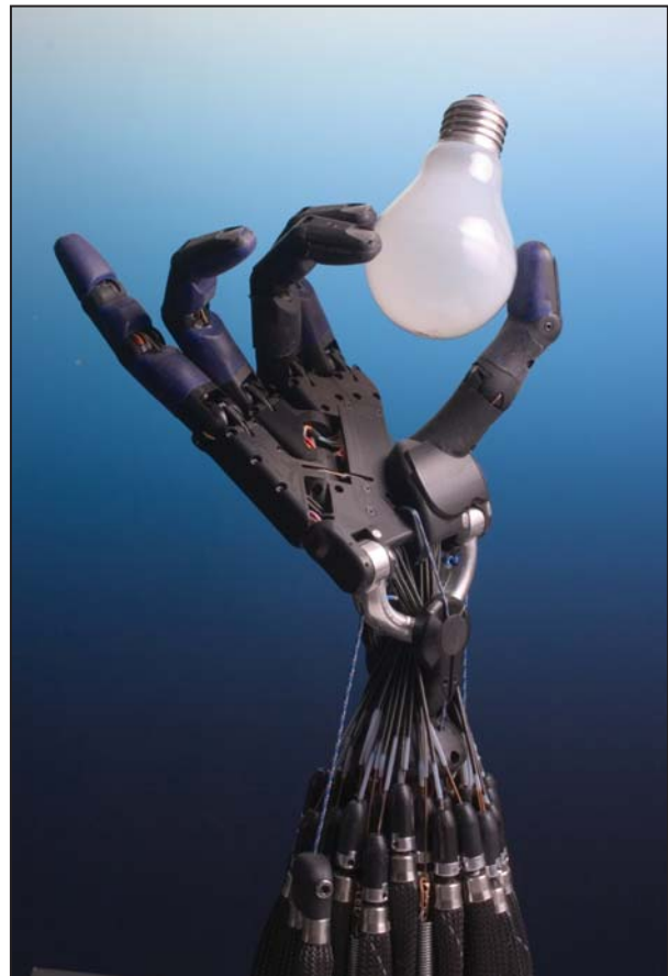
The Shadow robot hand system. Photo by Richard Greenhill and Hugo Elias/Shadow Robot Company, via Wikimedia Commons.
